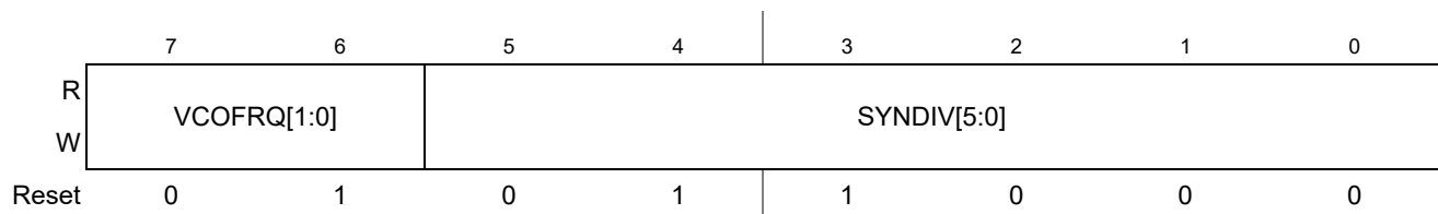
Figure 8-7. S12CPMU_UHV_V11 Synthesizer Register (CPMUSYNR)
