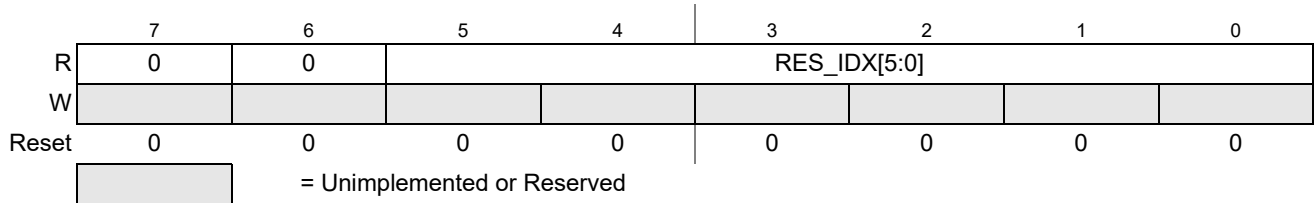
Figure 9-24. ADC Result Index Register (ADCRIDX)
