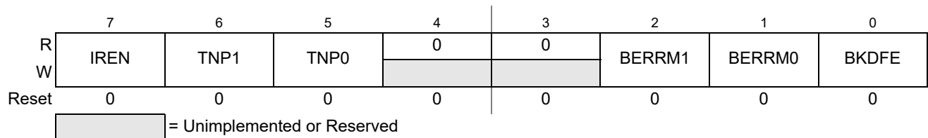
Figure 14-8. SCI Alternative Control Register 2 (SCIACR2)
