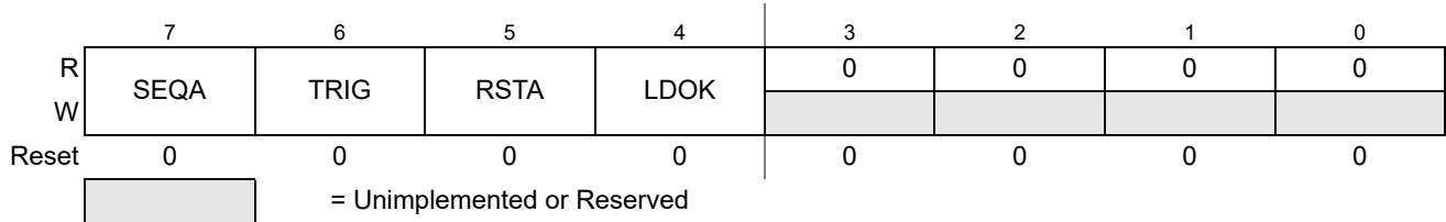
Figure 9-9. ADC Conversion Flow Control Register (ADCFLWCTL)
