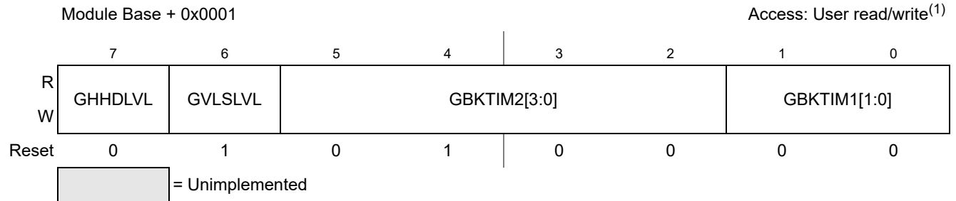
Figure 17-4. GDU1PHV1 Control Register (GDUCTR)
