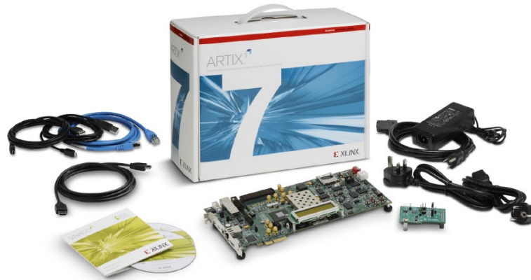
Artix-7 FPGA AC701 Evaluation Kit
