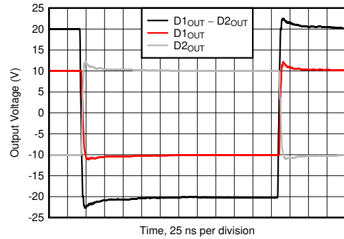
Figure 6-50. Large-Signal Pulse Response
