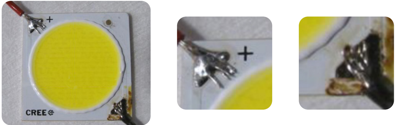
Figure 7: Left: Wires improperly attached to CX family LED, center: wires should not protrude beyond solder pads, right: excessive solder flux should be cleaned
